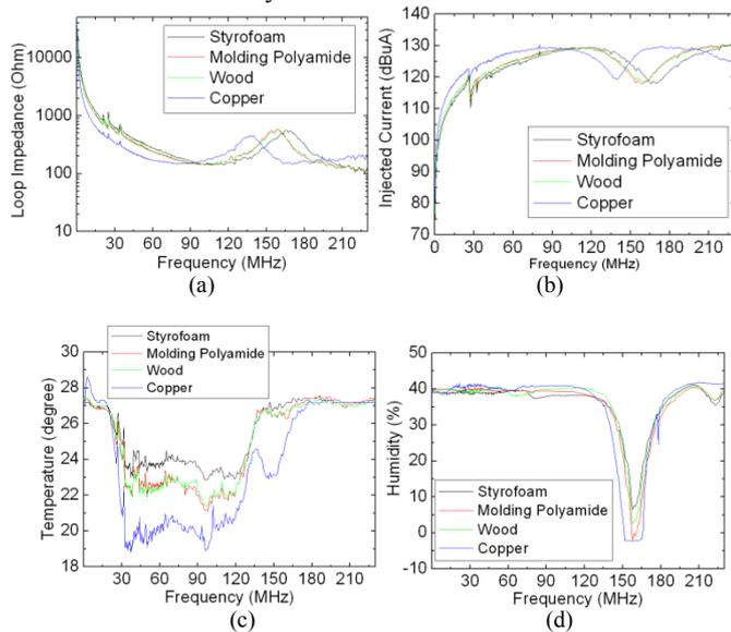
Fig 5. Results of thermo-hygrometer and supports with CDN (a) loop impedance values, (b) injected current, (c) temperature susceptibility level, (d) humidity susceptibility level
