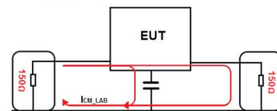
Fig 1. Conducted immunity test setup [10]
