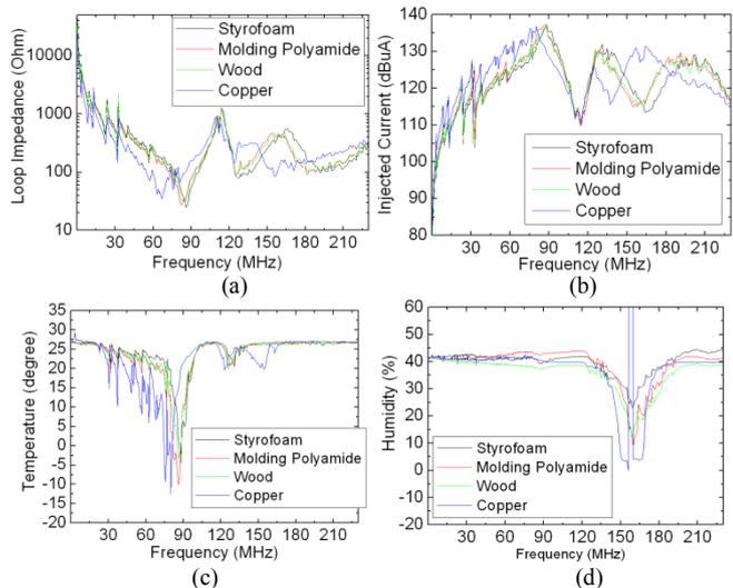
Fig 6. Results of thermo-hygrometer and supports along with connection to the mains without CDN (a) loop impedance values, (b) injected current, (c) temperature susceptibility level, (d) humidity susceptibility level
