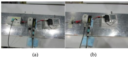
Fig 3. Conducted immunity test setups of the electronic thermometer (a) with CDN, (b) with mains without CDN
